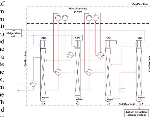
Fig. 2 Simplified flow diagram of the existing CD system
