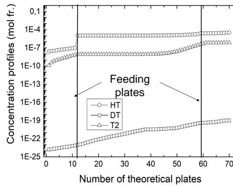
Fig. 7 Concentration profiles along the column 3
