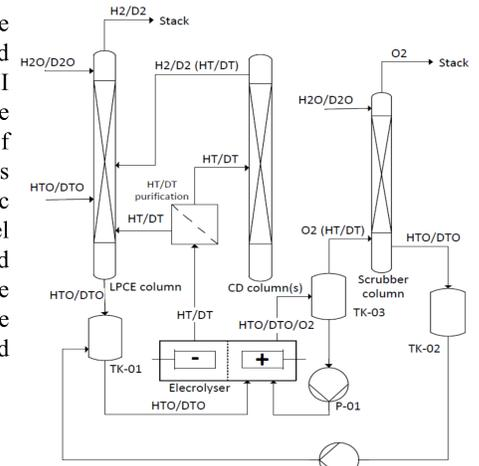
Fig. 1 CECE process connected to the CD system
