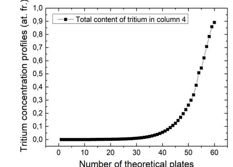
Fig. 12 Tritium profile along as-built column 4 (connected to modified column 3)
