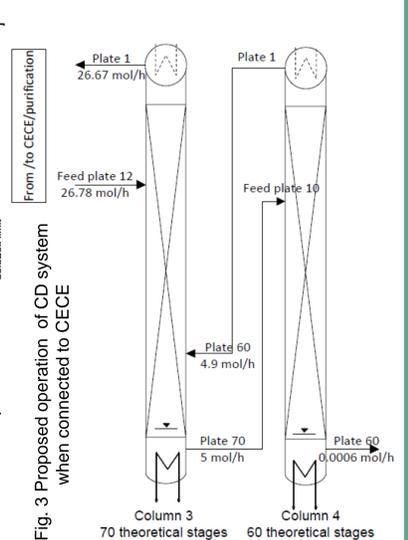
Fig. 3 Proposed operation of CD system when connected to CECE
