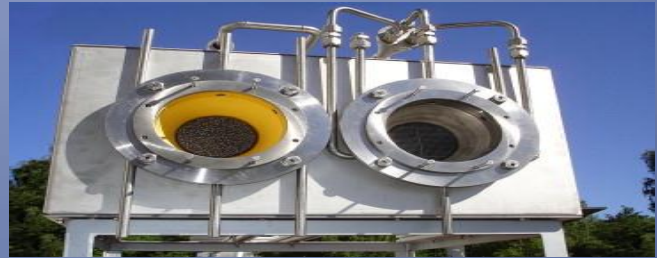
Fig. 2. Solar reactor with foam absorber in evaporator (left) and honeycomb in decomposer.
