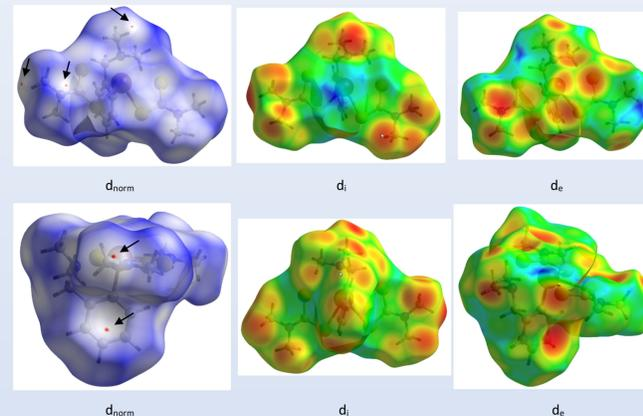
Figure 5. Hirshfeld surface for 4, mapped over  $d_{norm}$  over the range -0.010 to +1.367 arbitrary units (a. u.),  $d_i$  over the range 1.053 to +2.943 a. u., and  $d_e$  over the range 1.053 to +2.752.
