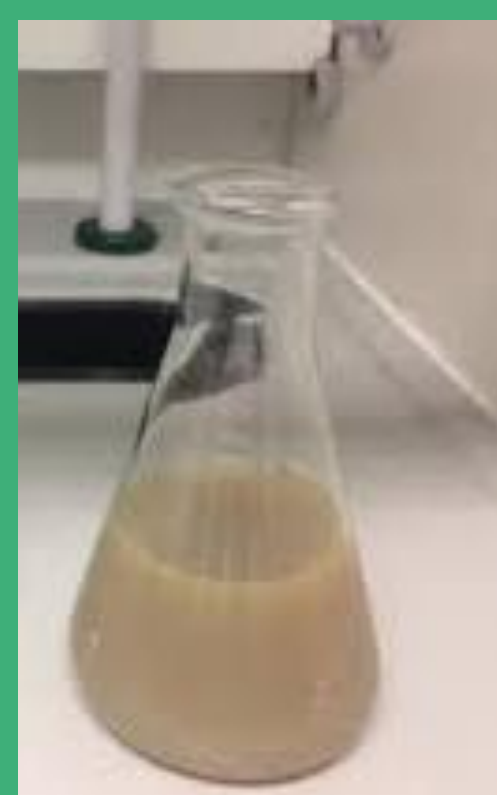
Grey suspension indicating successful nanoparticle formation.
