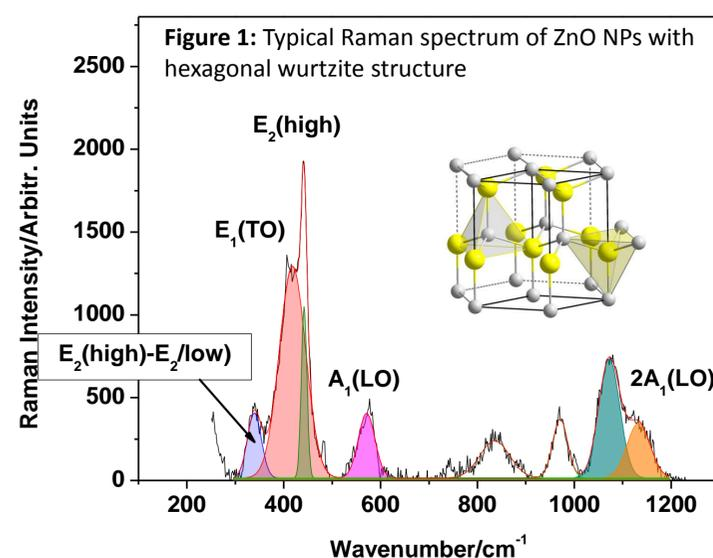
Figure 1: Typical Raman spectrum of ZnO NPs with hexagonal wurtzite structure
