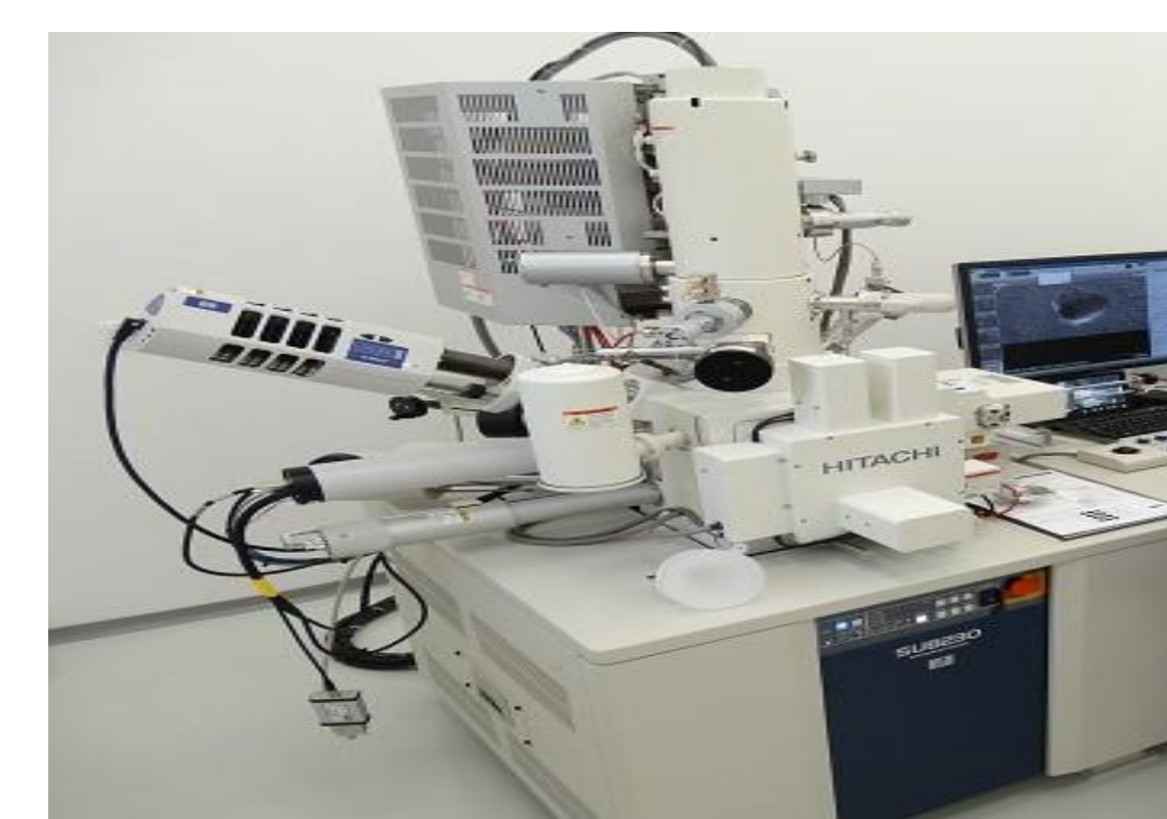
Scanning electron microscope (SEM) Hitachi SU 8230 Cold Field Emission, coupled with EDX analysis (Oxford Instruments, AZtec Software)
