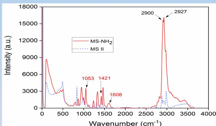
**Fig. 3** Overlapped Raman spectra of mesoporous silica (MS II) and amino silica (MS-NH<sub>2</sub>)
