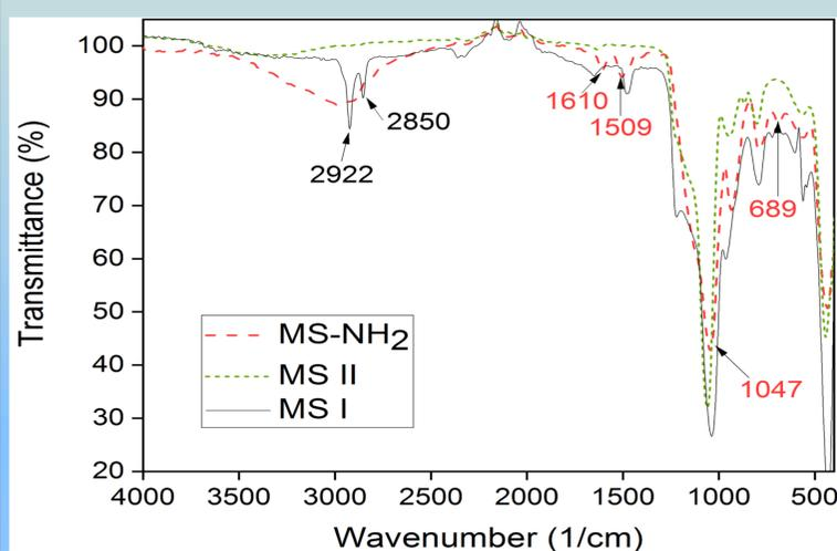
**Fig. 2** Overlapped FTIR spectra of mesoporous silica : (MS I), (MS II) and amino-silica (MS-NH<sub>2</sub>)
