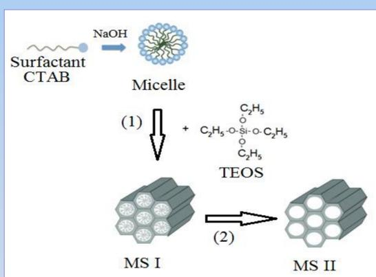
**Scheme 1.** Synthesis of the mesoporous silica nanoparticles (MS II)
