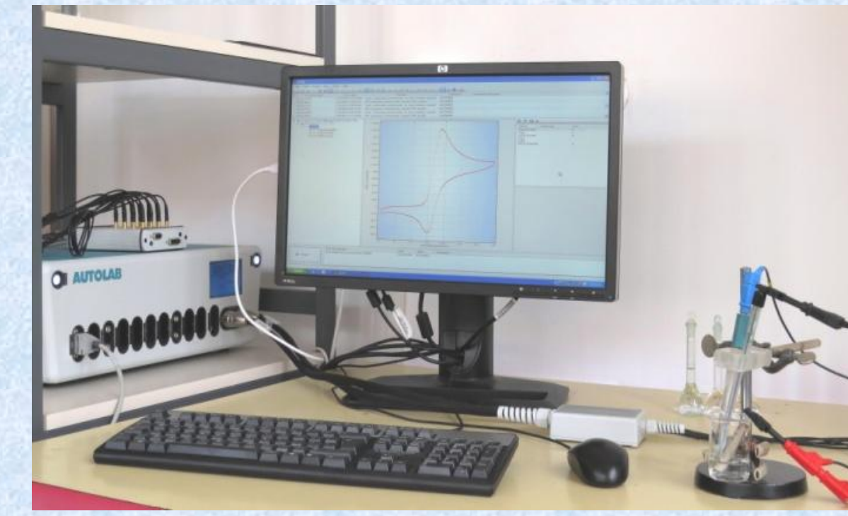
Experimental set-up for electrochemical measurements; Modified electrodes with triple-doped graphene
