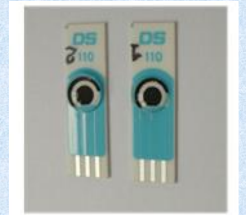
Experimental set-up for electrochemical measurements; Modified electrodes with triple-doped graphene
